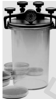
Figure 17 — Application of anaerobic gas generators for creation of anaerobic conditions in hermetically sealed vessels
