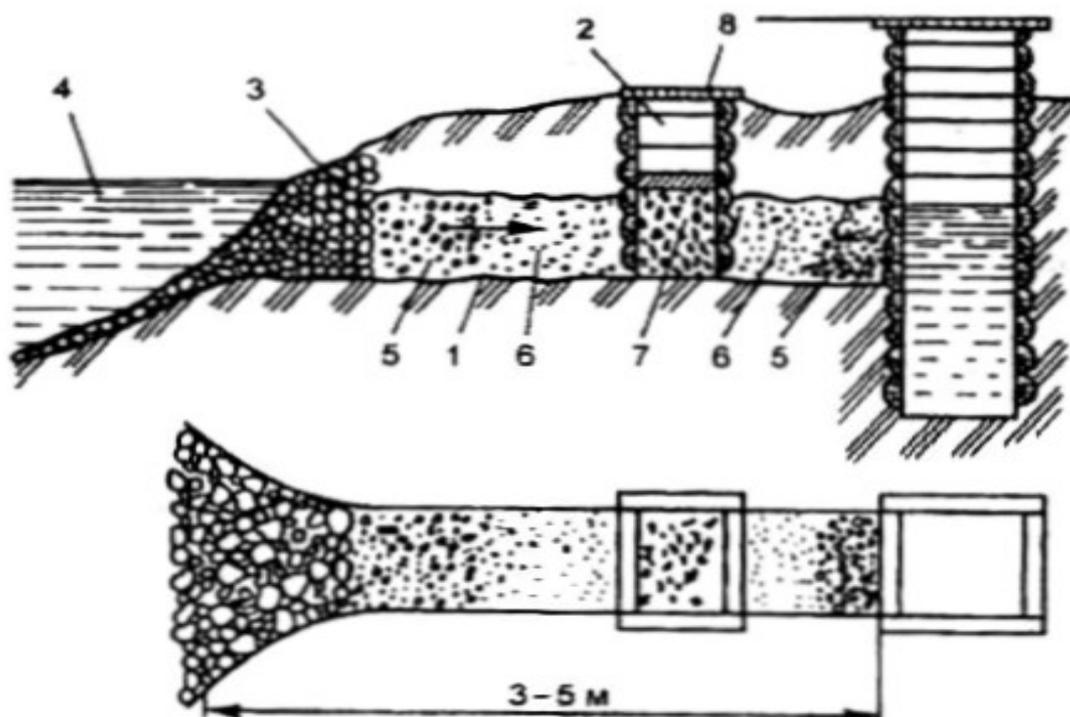
**Figure 1 — Well with filtration trench**
