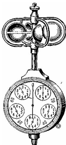
Figure 4 — Revolving-cup analyzer
