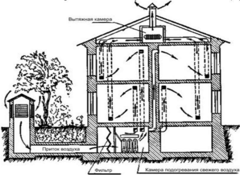
Figure 3 — System of a input and exhaust ventilation
