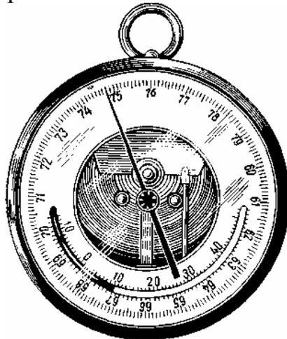
**Figure 7 — The Barometer-aneroid**
