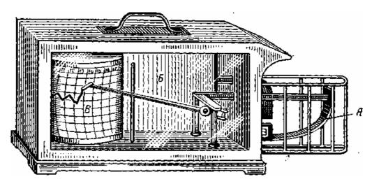
A — a plate filled with toluol; B — an arrow with a stylus; B — a rotating drum
