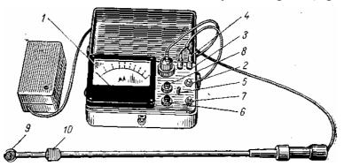
1 — a galvanometer; 2 — the switch of power supply;
