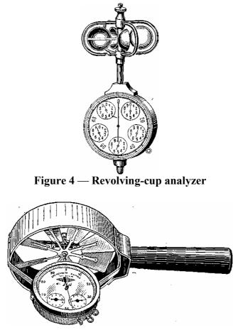
Figure 5 — Manual revolving-vane analyzer
