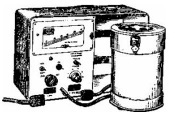
Figure 8 — Krotov's device for bacteriological research of air
