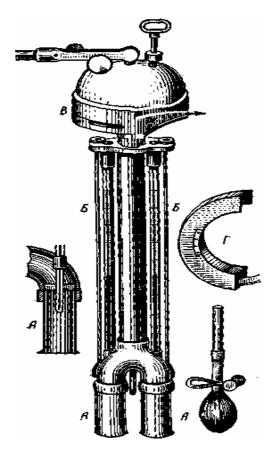
A — metal tubes in which tanks of thermometers are placed;B — thermometers;B — aspirator; $\Gamma$  — safety lock from wind; $\mathcal{A}$  — a pipette for wetting the damp thermometer
