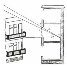
Figure 4 — Definition of a light angle and definition of aperture angle
